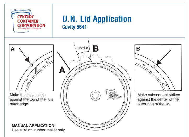
1. Position lid on top of pail. Using substantial force, strike the mallet against the top of the outer edge of the lid (see A above).
