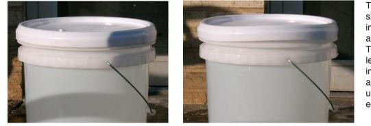
The far left photo shows the U.N. lid in the properly applied position. The photo at near left shows the lid improperly applied, as indicated by the uneven bottom edge of the lid.
